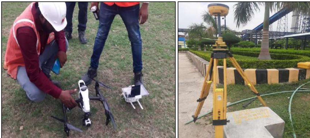
Fig 3 The Image of the Drone and DGPS used for the Canopy Survey
